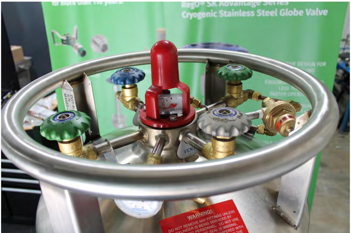
**For liquid cryogenic installation, it is recommended to use either brazed or back braze threaded end connections to avoid potential leakage through the threads that can occur during thermal cycling. RegO offers a diverse range of different end connections to help fit your specific installation needs.**
