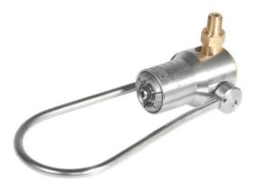
FasTest's G540 gas connector is simple to use with a no twist, no turn approach to filling. Simply connect onto your CGA 540 valve and lock into place with a forward movement of the bail handle roller actuator and you are ready to fill the industrial oxygen cylinder in a matter of seconds.
